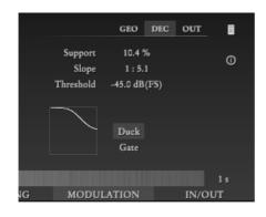
Selecting the envelope follower as modulation source enables a control field as shown on the side. The parameters in this field describe a function of decay time against envelope level: The support parameter controls a lower bound, the slope parameter controls the steepness of the dependency and the threshold parameter controls the level beyond which the effect sets in.
