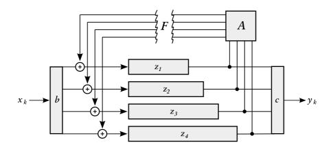
Figure 1: Block diagram of the signal flow inside ARIESVERB. Feedback matrix (*A*), input vectors (*b*), output vectors (*c*), input signal (*x*), output signal (*y*), delay lines ( $z_i$ ), scalar feedback gain, filters and saturation (*F*).
