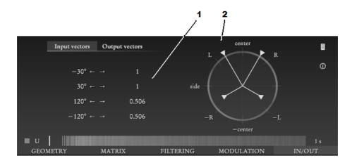
Numerical vector control: This field displays the bearing angle and the radius of either input- or output vectors, depending on which ones are currently active. Which bearing angles correspond to which stereo directions is summarized in the table below. A turn of 180° always corresponds to a phase inversion.
