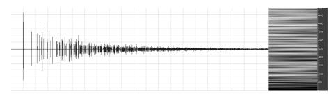
Figure 2: Impulse response of an ideal rectangular room, in time domain (left) and frequency domain (right).
